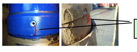
Note wear between new sub and sub run on the Jackdaw Sidetrack
